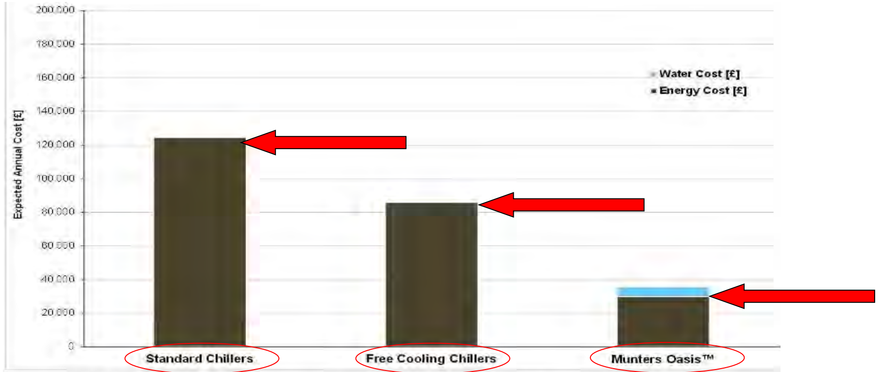
Figure 5.1.2. Total annual costs of energy and water consumed by the data hall.
