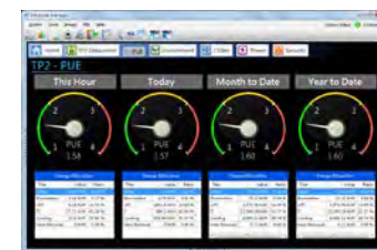
InfraSuite Manager (DCIM)
